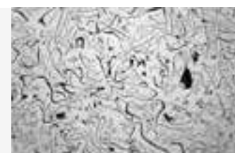
grey iron Excellent castability but brittle and not as strong
